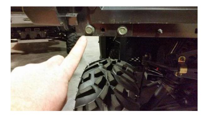
2) With bolts removed hold bumper into place and secure reusing the 10mm bolts. Leave bolts loose until all hardware is in.
