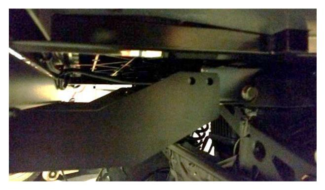
3) Using the supplied hardware secure bumper to frame and tighten all hardware. Installation is complete
