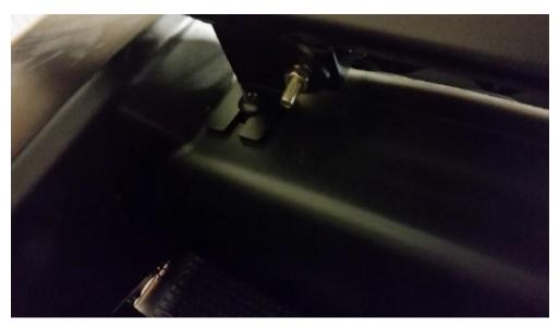
3) Using the supplied hardware bolt the lower bumper tabs to deflector plate. Tighten all hardware.
