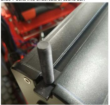
3) Install spacer onto T-bolts and secure T-bolts into place using (1)-8mm lock washer and (1)-8mm hex nut, per T-bolt. Lock into place approximating 12" apart.
