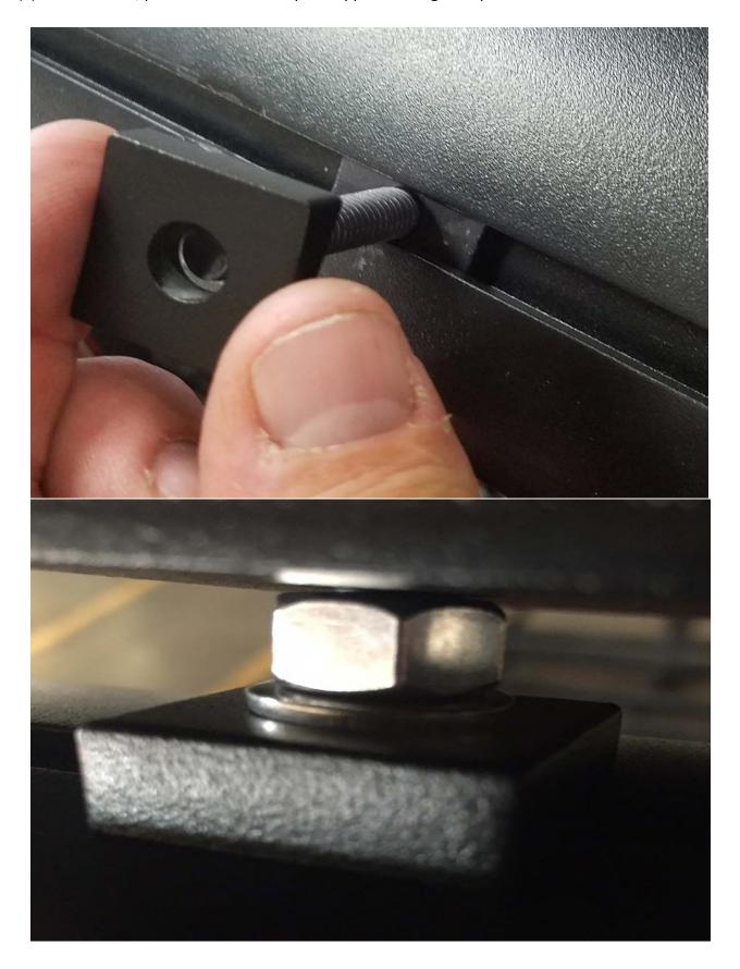
4) Mount the plates to the ROPS, using the provided 5/16" U-bolts and 5/16" Locking Flange Nuts, thru the slotted holes. Make sure the round holes are spaced at 12" to accommodate the T-bolt spacing from step 3. NOTE: T-bolt mounting holes should be towards the rear of the mower, i.e. the backside of the ROPS.
