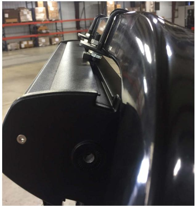
6) You are now ready to follow the instructions provided with the Wet Sounds Stealth Sound Bar for wiring and operation. Battle Armor recommends securing the cables to the ROPS with the included cable ties.
