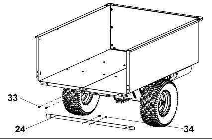
Attach Corner Gussets to Body and tighten all hardware.
