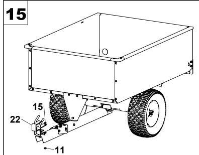
Slide Spring Loaded Hitch Bracket through drawbar and secure with hardware.
