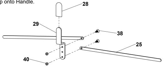
12 Slide Latch Bars into Tailgate retainers as shown. Align Handle with mounting hole on Tailgate.
