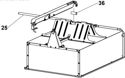
Slide Axle completely through Undercarriage; Swivel Clevis and Spacer must be captured by Axle.
